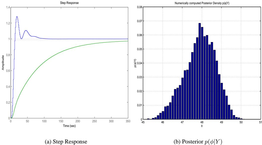
Figure 2: Figure (a): Achieved Step response on true system - faster response is closed loop response, slower response is open loop response. Figure (b): Posterior density  $p(\phi(K)|Y)$  of achieved phase margin given observed system response
